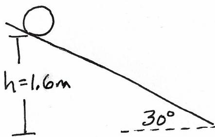
A hoop  $\neq$  a disk accelerate w/o slipping from rest down an incline of  $30^\circ$ . What is the speed of each at the bottom? The mass of each is 2kg and the radius is 0.25m.
